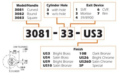
3080 Series Entry Trim accept any standard 1-5/32" diameter mortise cylinder with special MS $^{(0)}$  cam dimensioned as shown. Cylinders with MS $^{(0)}$  cams can be readily obtained from most cylinder manufacturers. See page SW-28 for cylinder make and trim ring information.
