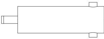
Thumbturn Tailpiece for Classroom Function Maxum® Deadbolt lock for doors 2 1/4" - 2 1/2" thick doors CT-F44
