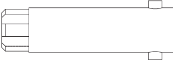
Thumbturn Tailpiece for Maxum® Deadbolt lock for 2 1/4" - 2 1/2" thick door (Includes: CP-281350 & CT-Y63) CT-F42
