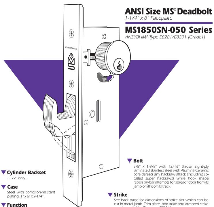
For hollow metal or wood sliding doors prepared for hardware according to the specifications of the American National Standards Institute, this MS® deadbolt provides maximum security and ease of installation. Its standard 1-1/2" backset dimension provides adequate clearance for the deep jamb "pocket" of many commercial and industrial entrances. Also useful for swinging doors closing against jambs too shallow for the 1-3/8" throw of the MS1850SN swinging door deadbolt.
