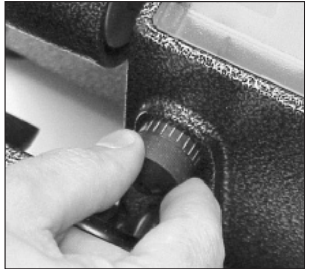
With the locking screw loosened, rotate the dial clockwise to increase cut depth or counter-clockwise to decrease as desired. (each mark is equivalent to 1½ thousandths of an inch change in cut depth).
