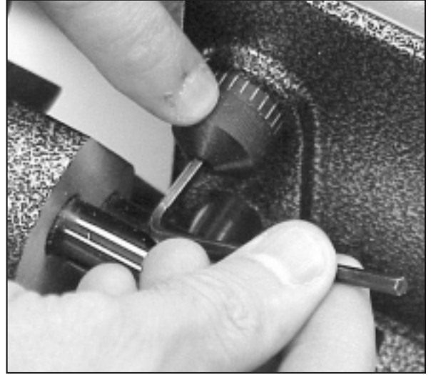
To change depth of cut, loosen the locking screw in the front of the Depth Adjustment Dial by turning it counter-clockwise about 1/2 of a turn.
