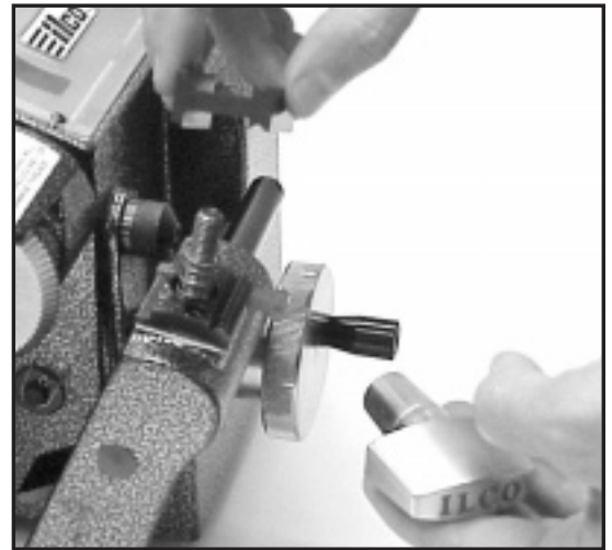
Option: Remove the upper vise and flip it over to use alternate position.
