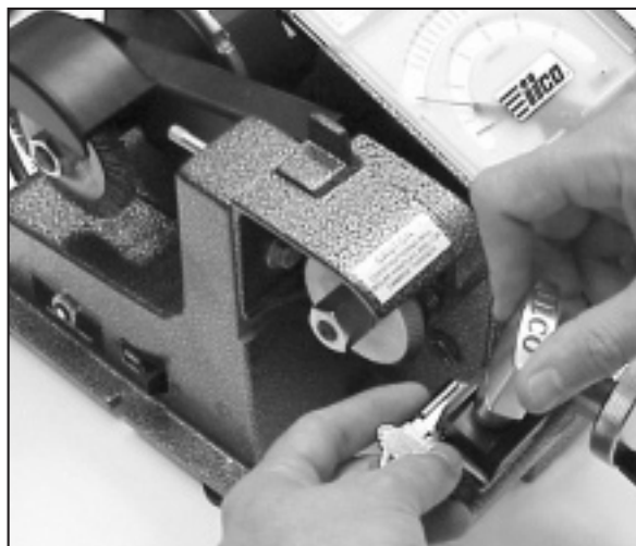
Align key using shoulder gauge or correct tip stop as required
