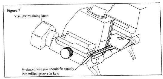
Before cutting this style of key, examine the key to see if there is a milled groove on either side. If so, then reverse the vise jaw and clamp the key using the V jaws. The key
