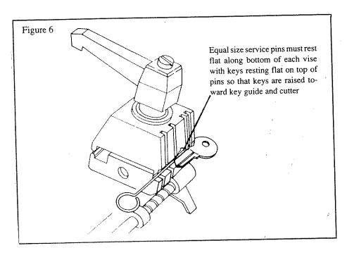
Some keys have a very narrow blade and therefore sit deep in the vise jaws with only part of the cuts showing above the vise. This makes it necessary to use the service pins to raise the key for proper cutting.
