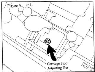
This machine is equipped with a carriage stop that prevents the carriage from moving all the way up to the cutter. When properly adjusted, it stops the cutter from grinding into the vise jaw. Such a condition could occur when reaching the tip of the cut key, and the carriage continues to move through its cycle.
