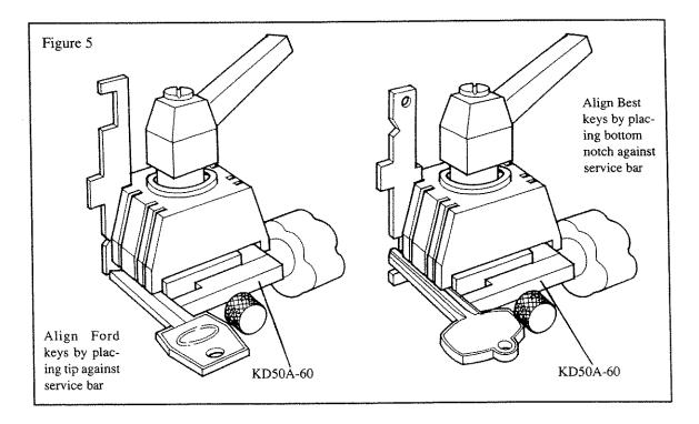
On keys without shoulders, the key setting gauge cannot be used. It is necessary to use the service bar to correctly position the key and the blank.
