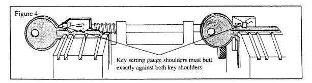
Insert the pattern key, left to right, into the left vise. Rotate the key setting gauge upward and set its left shoulder against the shoulder of the pattern key. Be sure the key is lying flat along the bottom of the vise. Secure the key by turning the clamp assembly clockwise.
