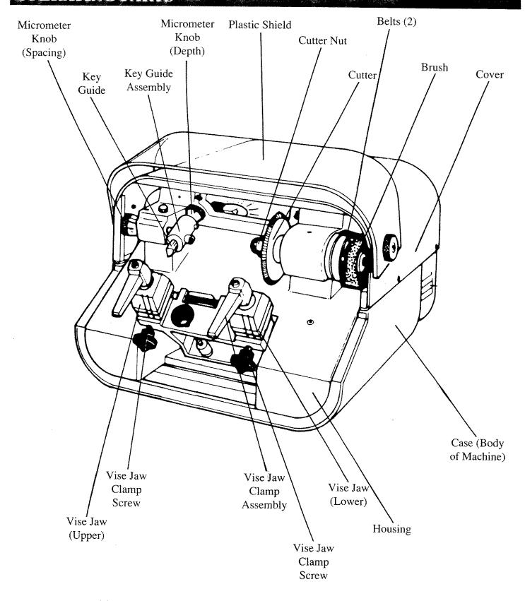
NOTE: On/Off power switch (KD50A-15) is not shown, but is visible on the left side of the machine.
