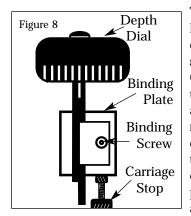
To adjust the cutter guide, loosen the binding screw on top of the cutter guide **slightly**. (see Fig. 7 & 8). Once you have loosened this screw, the depth adjustment dial can be rotated to the left (to decrease depth of cut) or to the right (to increase depth of cut). Again, proper adjustment will be achieved when the cutter
