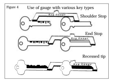
It is important that the key gauge prongs are in contact with both keys at the same time.
