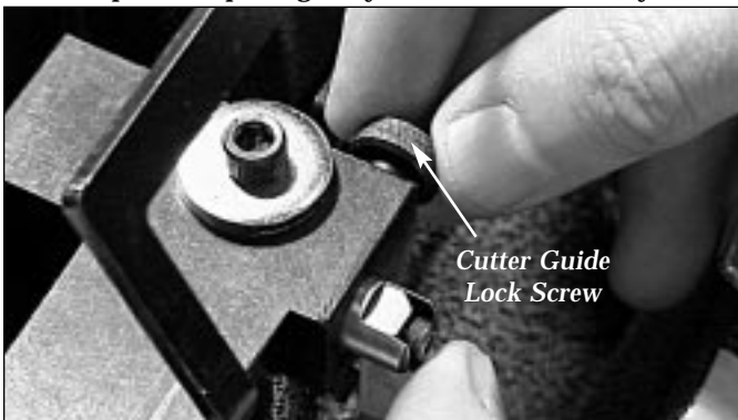
Figure 11 - Loosen Cutter Guide Lock Screw to allow guide to spring forward for code cutting
