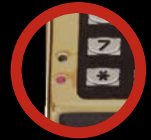
Flashing LED outside indicates the room is occupied or locked
