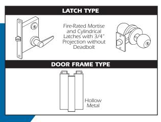
All 3/4" throw latches require 1/8" minimum door gap. Horizontal center line of strike must match center line of mortise latchbolt.
