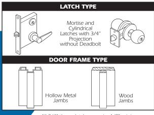
All 3/4" throw latches require 1/8" minimum door gap. Horizontal center line of strike must match center line of mortise latchbolt.
