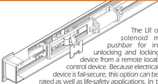
The LR option uses a solenoid mounted in pushbar for instantaneous unlocking and locking of the exit device from a remote location or access control device. Because electrical operation of device is fail-secure, this option can be used on fire-rated as well as life-safety applications. In the event of a power failure device automatically relatches. Requires the use of PS-LR Power Supply, which will power two exit devices. (Using an alternate to the PS-LR Power Supply will void warranty).
