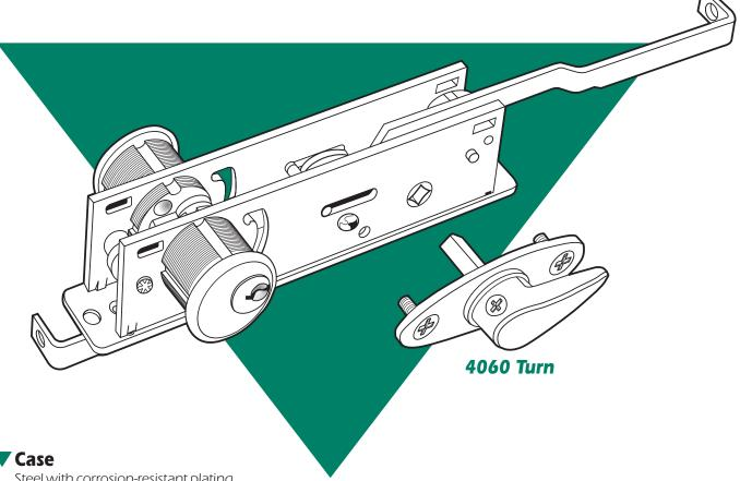
Steel with corrosion-resistant plating. 1" x 6" x 2"-5/8".
