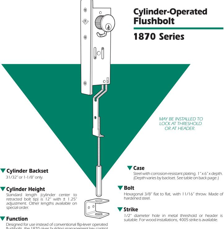
flushbolts, the 1870 gives building management key control of the inactive leaf of paired doors. Prevents casual locking of the inactive leaf by children or other unauthorized persons. Uses same basic overcenter action mechanism as MS® pivoted bolt locks. Recommended for installation at both top
