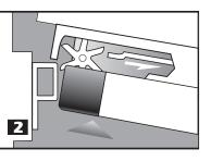
[1] When door closes, the interlocking noseguard and Starwheel bolt close around the strike. The deadlocking slide springs over, locking the Starwheel bolt to the strike. [2] When pushbar is depressed, the deadlocking slide moves back, allowing the door to unlock from the strike. This unique interlock provides solid security and prevents jamb spreading.
